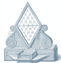
Fig. 750.—Cooke and Wheatstone's Five-Needle Telegraph.
